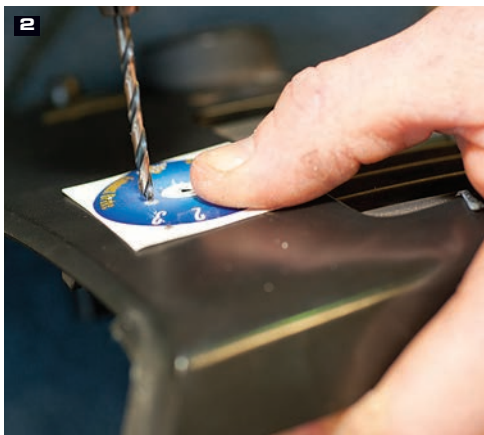
1) Run the wires from the control switch from the engine compartment into the cab on the driver's side. Then carefully pop loose the upper left dash panel. 2 & 3) Drill out the center hole (switch shaft) and smaller outer hole (for lock pin) using the BD VVB decal as your guide.
