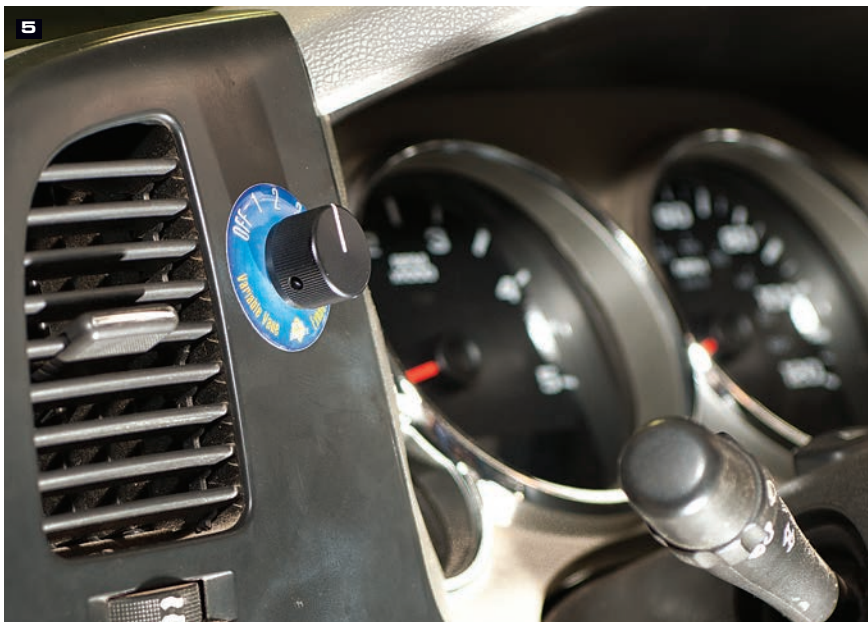
5) Control knob placement high on the dash makes it easy to see and access. Three stages of exhaust braking/downshifts are available with the turn of the selector.
