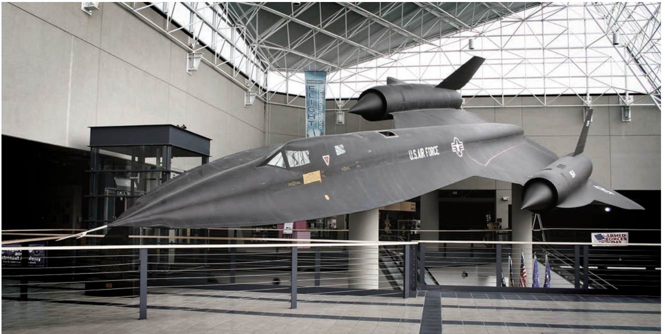
Above: The Lockheed SR-71A Blackbird is a high-speed reconnaissance plane designed to outrun the U-2 spy plane. Its maximum speed is still classified, but its cruising speed is 1,320 mph. Below: Snow-covered Rocky Mountains from historic Route 40 in Colorado.
