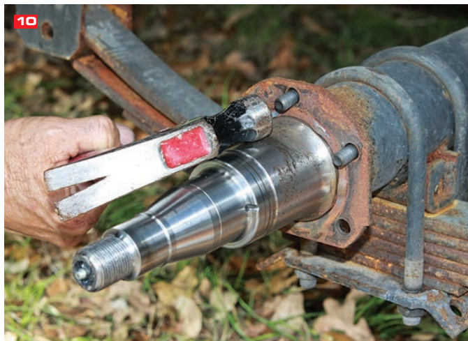
8) Remove the old electric brake assemblies, clean and prep area for installation. 9) Hub and rotor is held in place to ensure a proper fit before bolting to the axle. 10) Old studs that held the electric brake assembly are removed because they are too short for the new hardware.
