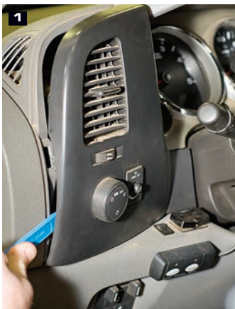
1) Run the wires from the control switch from the engine compartment into the cab on the driver's side. Then carefully pop loose the upper left dash panel. 2 & 3) Drill out the center hole (switch shaft) and smaller outer hole (for lock pin) using the BD VVB decal as your guide.
