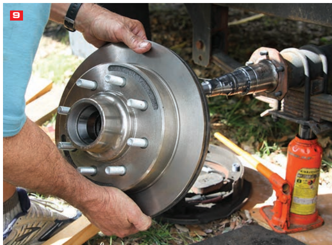
8) Remove the old electric brake assemblies, clean and prep area for installation. 9) Hub and rotor is held in place to ensure a proper fit before bolting to the axle. 10) Old studs that held the electric brake assembly are removed because they are too short for the new hardware.
