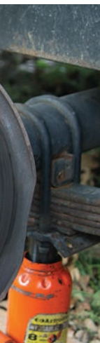
8) Remove the old electric brake assemblies, clean and prep area for installation. 9) Hub and rotor is held in place to ensure a proper fit before bolting to the axle. 10) Old studs that held the electric brake assembly are removed because they are too short for the new hardware.
