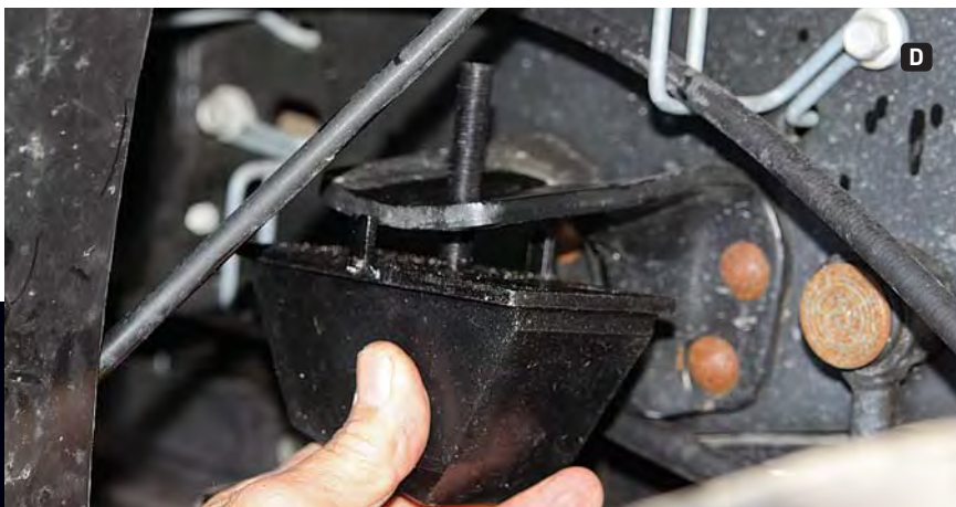
C) A pry bar is used to remove the factory contact pads. D) Stable Load pads are installed in the frame bracket with the anti-rotational key facing outward.
