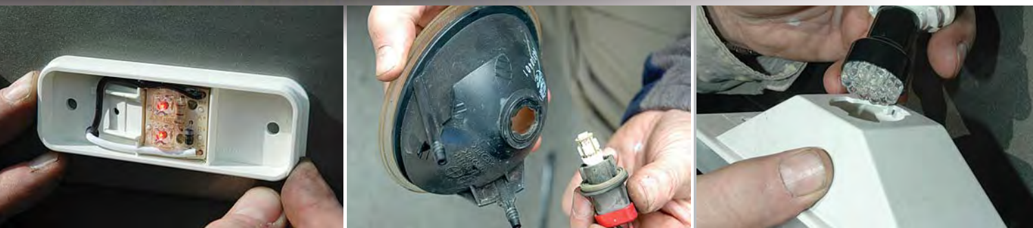
From left: Optronics replacement side markers for both red and amber featured light-emitting diodes that were actually the correct color. The Jirah 1330 B45 R5 Extreme with 13 LEDs was a good fit and did produce more light than the original incandescent bulb. Some replacement bulbs were too big to fit the housings.
