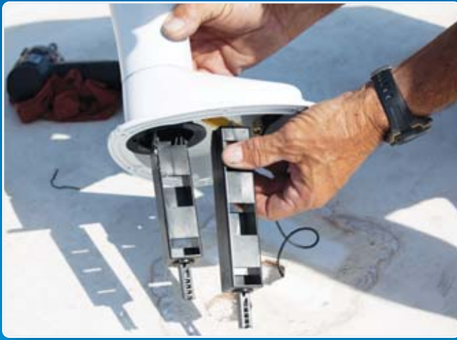
Installation of the supplied longer connector is as simple as slipping it on over the stock adjustable connector.
