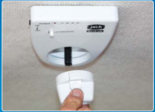
Press the button located on the side of the rotation knob. Then press it onto the adjustable connector.
