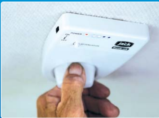
Rotate the antenna until you see the signal meter indicator lights turn on.
