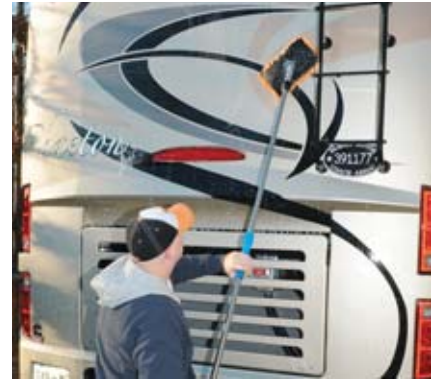
The Griot's microfiber wash pad is another cleaning tool that's easy on the paint. When attached to the company's very good extension pole it was easy to reach the entire coach and the microfiber pad won't scratch the paint like synthetic brushes can. Since the pad is not as thick as a brush, it makes cleaning around slideouts and awning arms tougher. Overall we still prefer the boar's hair brush.
