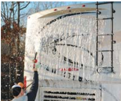
After wetting down the coach, we mixed the DP shampoo in the Autogeek foam cannon and applied it to the motorhome. This combination was by far the best at creating thick foam, which helps to float away contaminants and protect the paint from swirls.
