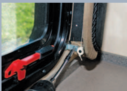
STEP 3. We used a cordless drill and a long flexible bit holder to make accessing the screws as easy as possible. Other locations require a screwdriver depending on available space.
