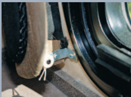
STEP 2. First you will need to locate all the L-brackets that secure the valance to the wall and remove them one by one. Sometimes there are some hidden brackets so look carefully before you try to remove the valance.
