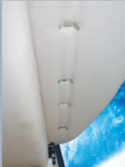
STEP 22. Release the old shade from the factory clips above the dash. Since the old shade was a one-stage unit, it only had four clips. Before installing the new, heavier two-stage Day/Night shade we added several more clips to carry the extra weight.
