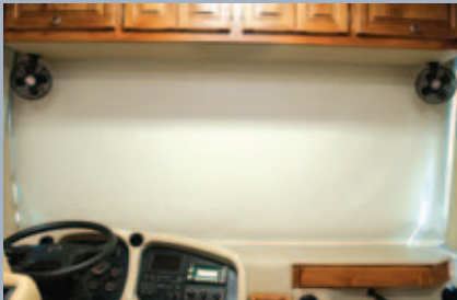
STEP 21. This coach came from the factory with the MCD electric front night shade but it was not the same two-stage Day/Night shade as the others we installed. We removed the old windshield shade and replaced it with the newer model that includes electric operation for both shades as well as programmable limit switches that prevent the shades from closing too far when the engine is running. This is a long and heavy shade so this was by far the most difficult one of the project, requiring two people.
