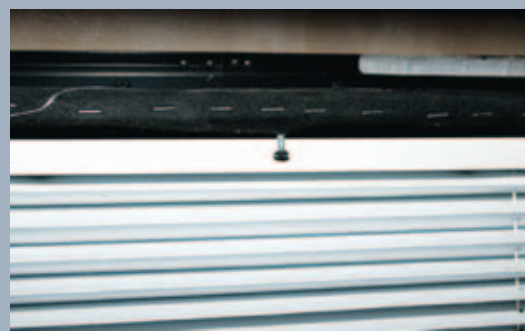
STEP 5. On this coach, each shade had a single screw in the middle that helped hold the center and, of course, it too has to be removed.
