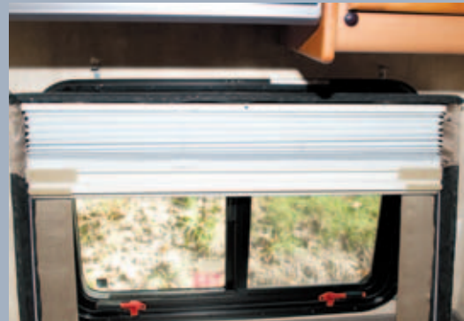
STEP 4. After removing the valance, flip it over so you can see the back and determine how the shade is attached to the valance.
