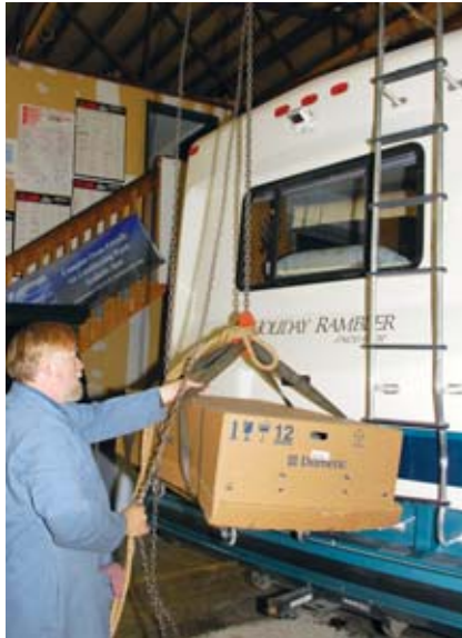
STEP 1. You may not have considered how you're going to get your new A/C unit on the roof, but it's something to seriously think about before ordering it. These units are large and heavy (about 100 pounds), so if there's no practical way to get it up there safely, consider leaving the job to professionals. Imperial General Manager Ed Hall uses straps and a chain hoist attached to the shop's roof beams to move the unit to the roof.
