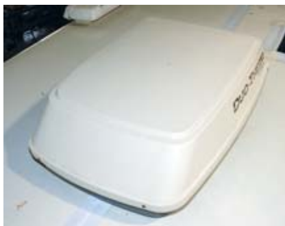
STEP 2. The original Dometic Duo-Therm unit did its job for many years, but stopped blowing cold air eventually. Unfortunately, it is not cost-effective to recharge these older units with new refrigerant, so they should be replaced.
