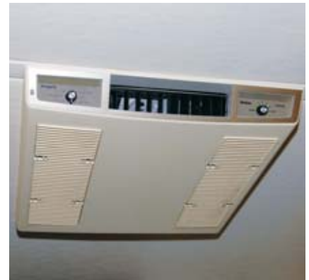
STEP 4. The job begins with removing the old cover, as this will provide access to the wiring harness and fasteners that clamp the A/C unit to the roof.
