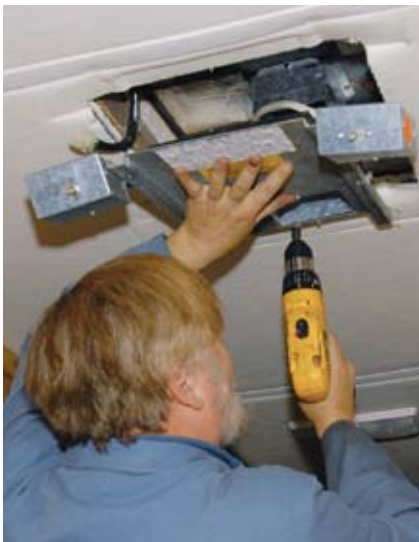
STEP 8. Hall begins removing screws that hold the motorhome's sheet metal work in place, then holds it with one hand as the last few screws are removed.
