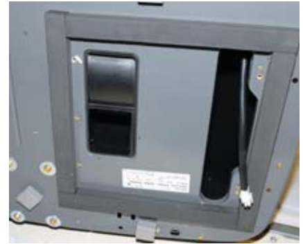
STEP 3. The underside of the A/C unit reveals the ducting, foam gasket and wiring harness with male connector. Many new A/C units are available as a direct replacement for your old one, but be sure that the male connector on your new unit is compatible with the female receptacle in your RV. If not, you'll either have to order another unit that is compatible, or rewire the receptacle in your motorhome to accommodate the new harness. It's better to find out now than after you've installed the unit.
