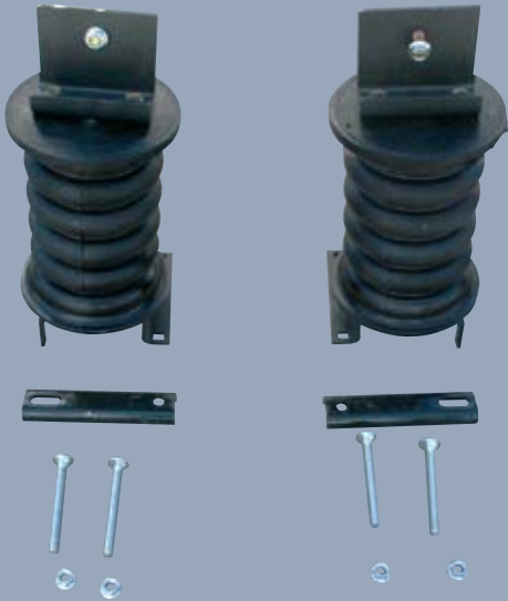
The front Ford F53 kit comes with brackets and hardware and sells for $655. Labor time is about one hour.
