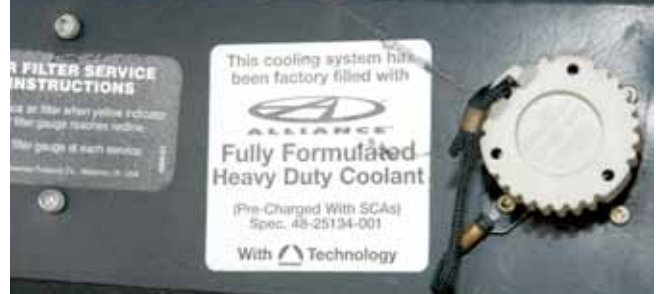
This 2008 Freightliner chassis has a label that indicates exactly which type of coolant was initially installed. Alliance is a fully formulated coolant that uses nitrates for cylinder wall pitting protection; therefore it should be tested with two-way test strips.
