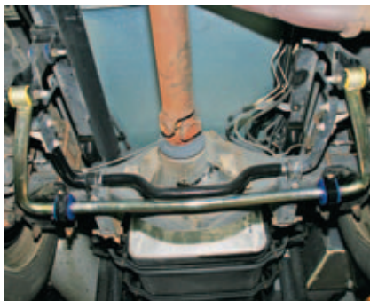
The larger Roadmaster rear bar encircles the stock Ford bar and more than doubles roll resistance.
