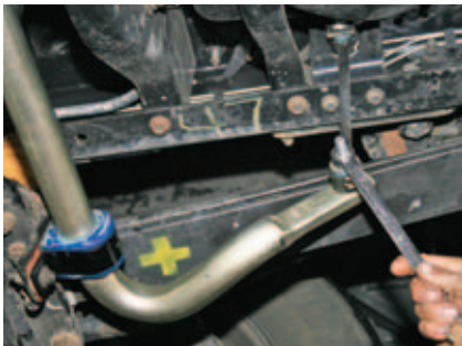
Roadmaster front bar is thicker than stock bar and utilizes stock frame linkage.
