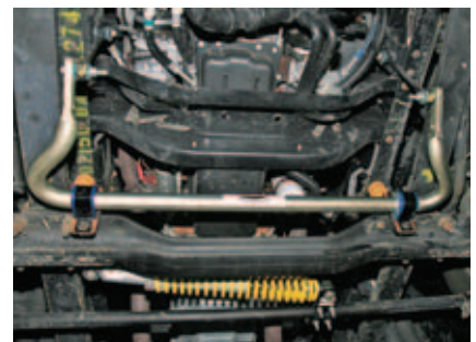
Roadmaster front anti-sway bar is fitted forward of the axle while the Reflex Steering Stabilizer is attached to frame behind axle and to tie-rod end (center, rear).
