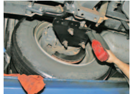
Roadmaster steel brackets are fitted below rear axle, using existing U-bolts.
