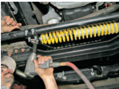
Position of tie rod bracket determines neutral position of stabilizer.
