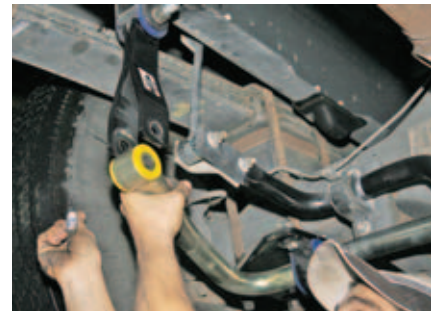
Polyurethane bushings permit less flex between bar and frame brackets.
