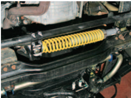
Reflex Steering Stabilizer, bolted to frame (right) behind axle and to steering tie rod (center), exerts spring pressure to re-center steering and dampen steering motion.
