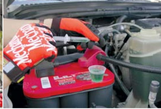
Polaris Laboratories offers an easy-to-use test kit for taking small samples of your coolant to use with its test strips.
