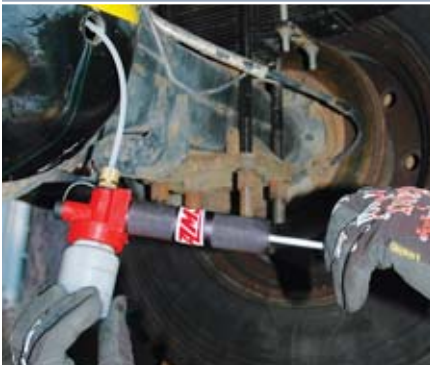
Amsoil's Oil Analysis Pump Kit (Part #G-1206) is a simple and clean way to take samples out of the rear axle.
