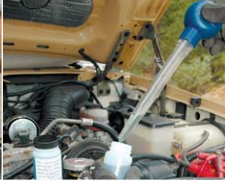
A turkey baster is an easy way to extract a sample of coolant from your radiator for lab analysis.
