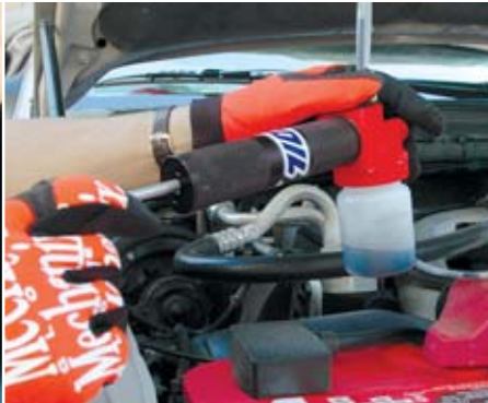
The Oil Analysis Pump Kit (Part #G-1206) from Amsoil uses a long tube, which is inserted down the dipstick tube. Oil or lube is pumped directly into the test jar.
