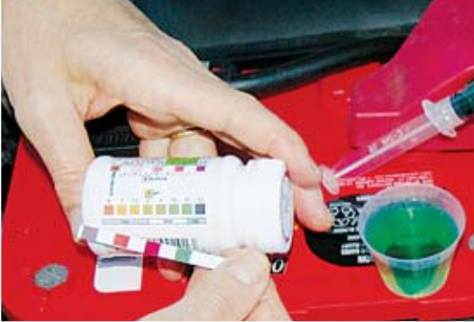
The Polaris Quik-Chek can tell you the freeze point, pH, and concentration of molybdate and nitrite, which in turn will determine the number of supplemental coolant additive (SCA) units per gallon in the system.
