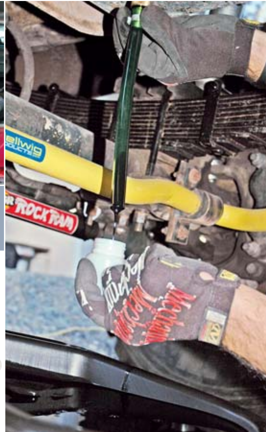
The Femco No-Spill System uses an adapter in the oil pan and a drain plug with a valve that allows all or just a little oil to flow out. No drips. No mess. No oil running down your arm.
