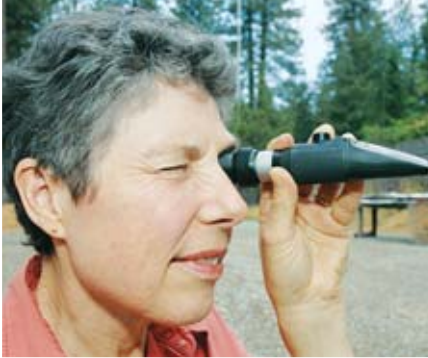
A refractometer is a simple way to determine the freeze point protection for the mixture you have.
