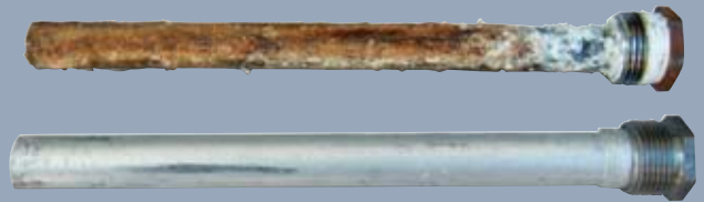
The top anode rod is in obvious need of replacement. The rod is more prone to corrosion than other metal tank parts.
