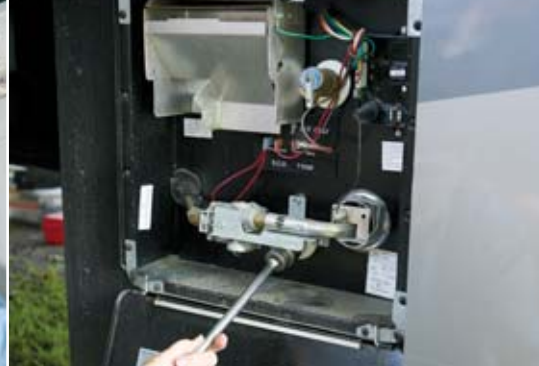
After bypass valve is set, water drain plug should be removed to empty tank.
