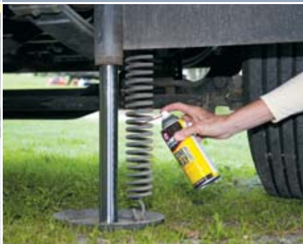
Hydraulic jack rams should be lubricated if extended while coach is in storage.
