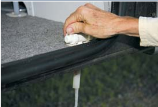
Low-point drains are helpful but don't ensure that all water is removed. Antifreeze should be used.
