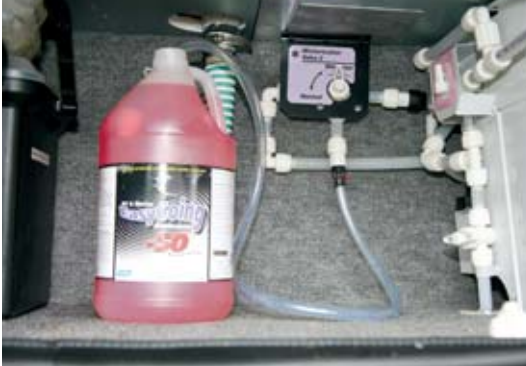
Winterization is easy with a built-in system for pumping antifreeze into water lines.
