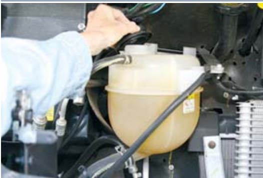
If the engine is due for a coolant change, the best time is before winter lay-up.
