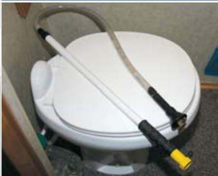
Without an in-tank cleanout fitting, a spray wand should be used via the toilet to flush black tank.
