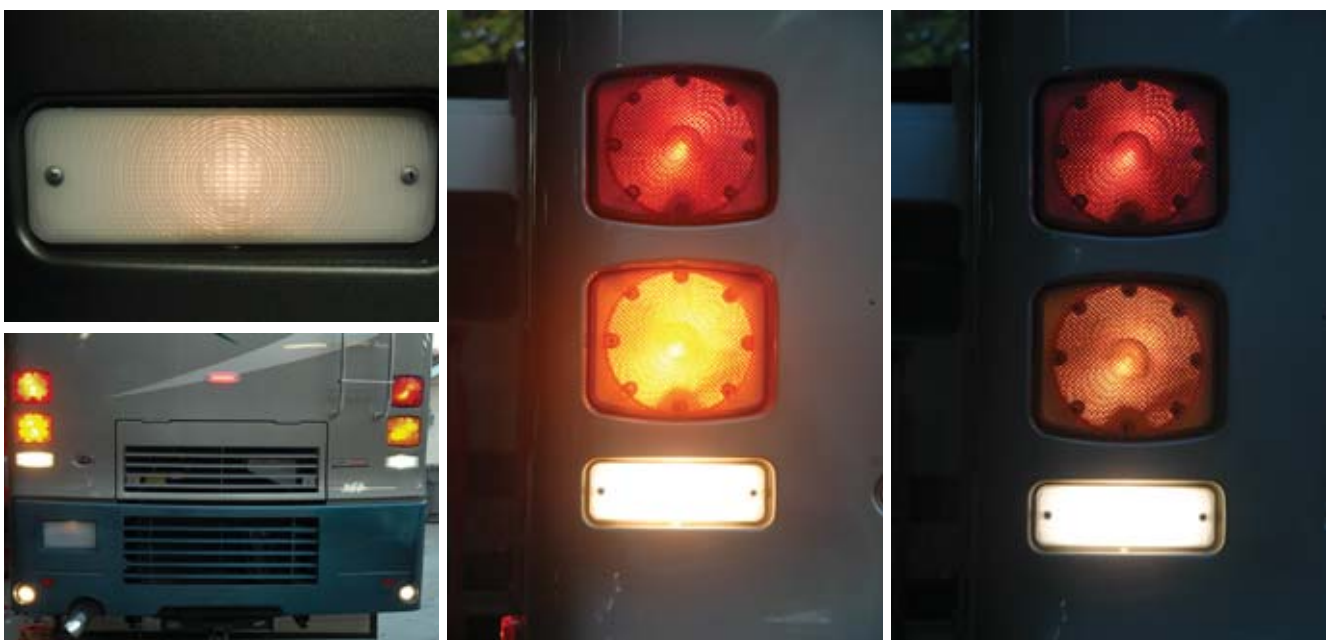
Clockwise from left: Using an LED replacement bulb in the backup light proved an ineffective choice. OEM incandescent bulbs in turn-signal, brake, running and backup lights were significantly brighter. When we used LED replacement bulbs in the same applications they proved to be a huge disappointment. You can see the difference at the rear of the coach — on the left are OEM bulbs and on the right are LED replacement bulbs.
