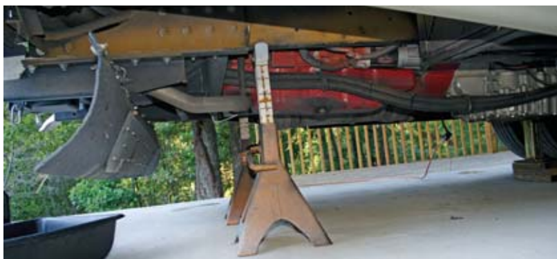
Since this procedure requires you to be under the motorhome you should not rely solely on the coach's jacks. We used a heavy-duty pair of stands and placed them directly under the frame rails. Since this is a safety issue it is a step that you cannot bypass. In case the coach jacks fail you need something that can carry the rear axle weight, which is 20,000 pounds on this coach.
