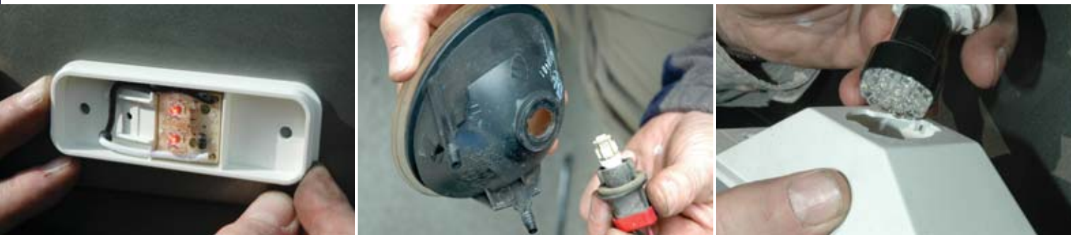
From left: Optronics replacement side markers for both red and amber featured light-emitting diodes that were actually the correct color. The Jirah 1330 B45 R5 Extreme with 13 LEDs was a good fit and did produce more light than the original incandescent bulb in the docking light. Some replacement bulbs were too big to fit the housings.
