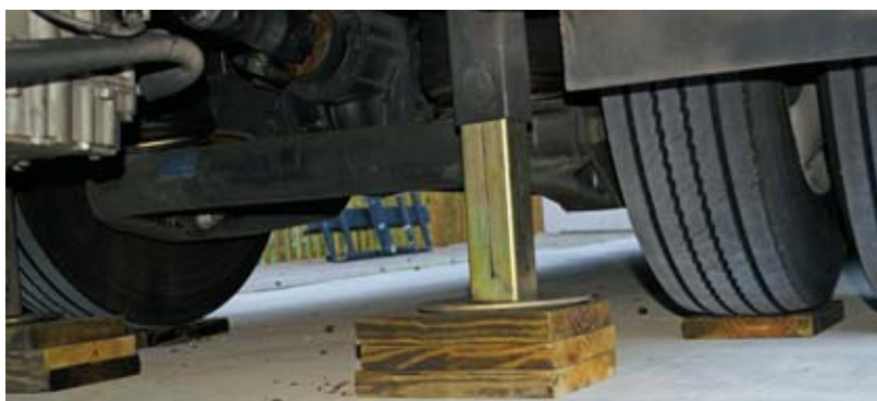
In order to raise the rear of the coach we placed several wood "jack pads" under the coach's leveling jacks and lifted it to the necessary height to allow easy access to the transmission pan.
