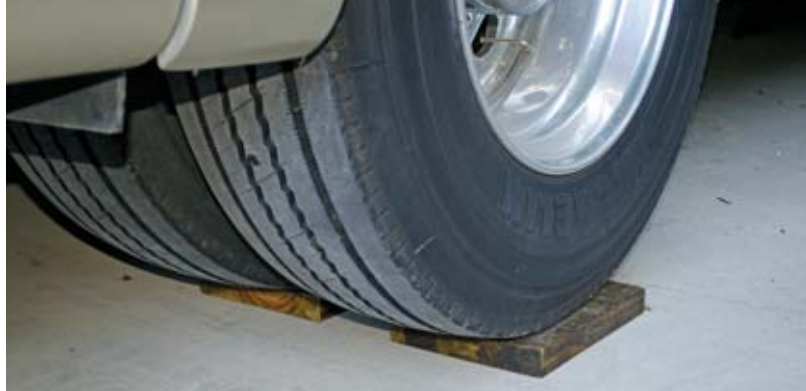
We raised the rear of the coach by 1.5 inches by driving it on to 2-by-10-inch wooden blocks. This makes access under the coach easier. Just make sure the blocks are wide enough to support the entire footprint of the tire to prevent damaging it.
