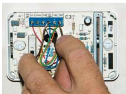
Jumper leads can be used to bypass several controls in motorhomes. Be sure to check the service manual to avoid damaging control boards when using jumpers.
