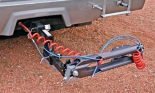
The Sterling tow bar is easy to handle and collapses for storage behind the motorhome. A drop receiver is used to lower the bar to a level position.
