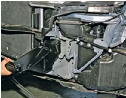
The mounting bracket was a precise fit for the CR-V, inserted into the car frame in place of the bumper core.
