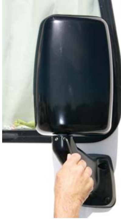
8. With the primary driver sitting behind the wheel, loosen the Allen screws and adjust the mirror head into the desired position.
