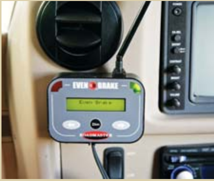
The monitor reflects the status of the Even Brake and signals when brakes are applied.
