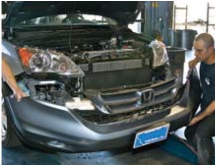
The Honda CR-V grille/bumper fascia was easily removed for installation of the mounting bracket for towing.
