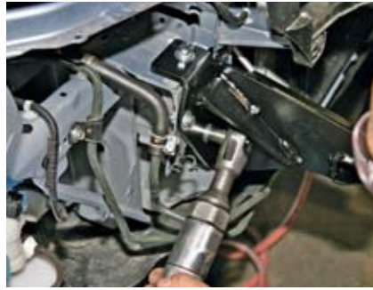
Original Honda fasteners were used when bolting the Roadmaster mounting bracket to the frame.
