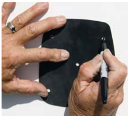
2. Use the supplied Velvac gasket as the template for drilling the new holes.
