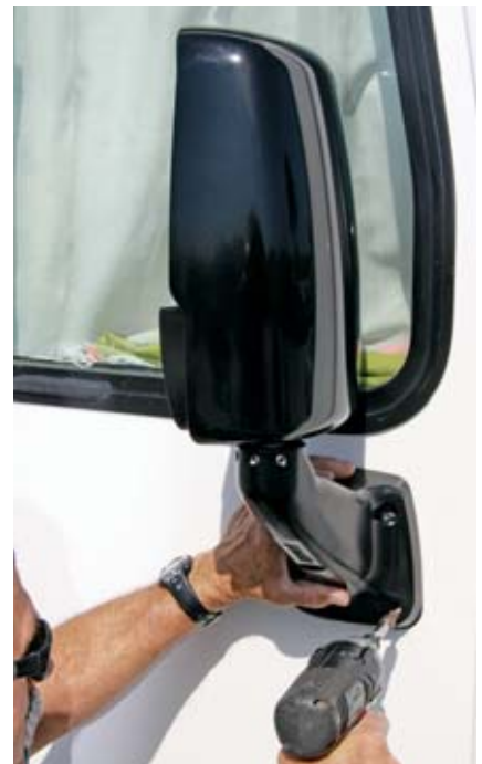
6. With one hand, hold the mirror in place and install the supplied screws.
