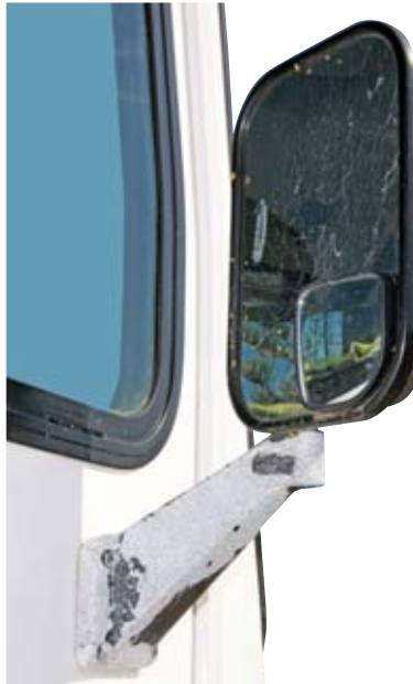
1. The old Velvac mirror lacked adequate size — especially with the aftermarket stick-on blind spot mirrors.
