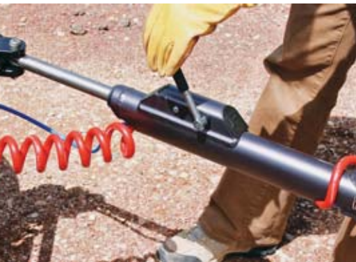
Roadmaster's Freedom Latch eases the release of tow bar arms even when they're under pressure in a bind.
