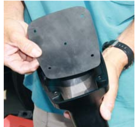
4. Peel and stick the Velvac gasket and place onto the new mirror base.
