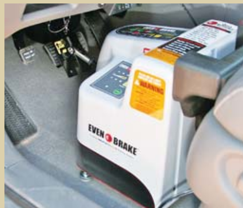
An air compressor and inertia-sensing controls are contained in the Even Brake unit, which is attached to the brake pedal before each towing session.
