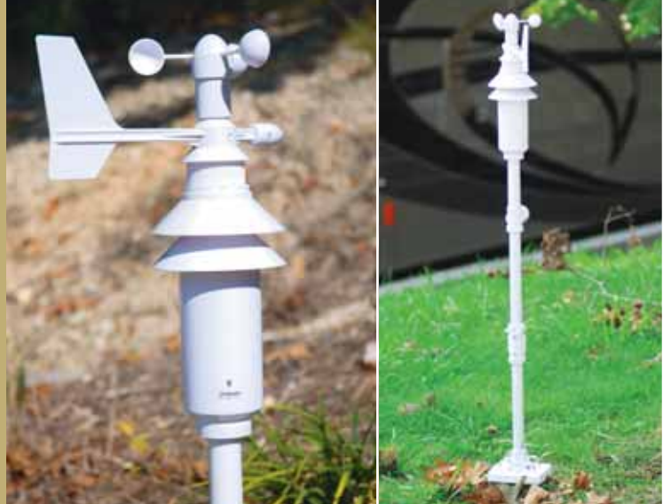
The Oregon Scientific WMR100 weather station comes with an LCD monitor and outdoor gauges. The rain gauge never needs to be emptied and the combination temperature/humidity/wind speed/wind direction sensor is easy to set up in camp. An updated version of this unit was recently released, which features separate sensors for rain, temperature/humidity and wind speed/wind direction.
