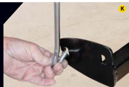
K) Fastgun turnbuckle end slips into the provided hole in the tie-down insert before adjusting tension. L) Rubber O-ring is used to make final adjustments. When the lever is locked the space between the O-ring and the turnbuckle body should be 1/4-inch.
