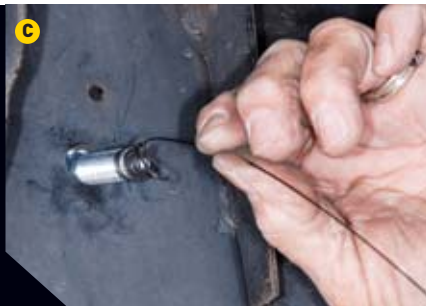
A) Front brackets are bolted to frame using existing holes; fit is very precise. B) Tie-down inserts are slid into frame brackets and held in place with pins. C) Fish wire is used to thread bolt through frame with restricted access. D) Painter's tape is used to prevent bolt from slipping out of hole while second bolt is fished through frame.
