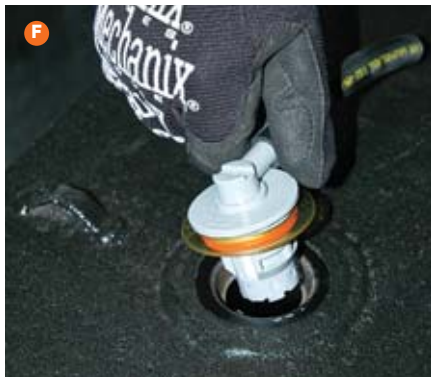
D) A new float arm was attached to give an accurate fuel level calibration for the larger tank. E) Transfer Flow replaces the twist-lock compression seal with a new O-ring and gasket, and a top-sealing ring that is attached with six nuts over studs. F) Two new rollover valves were fitted.
