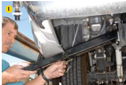
E) A piece of 3/8-inch tubing is wrapped around emergency brake line using a cable tie. F) Tubing prevents the emergency brake line from rubbing against the bracket. G) Four holes are drilled into the hitch receiver side plates. H) Rear brackets are bolted to hitch receiver side plates. Washers can be used if there's an interference problem with the exhaust tailpipe. I) Insert slides into rear bracket and is pinned in place. J) Fastgun turnbuckles must be assembled before positioning.
