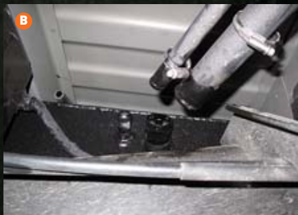
A) Though it may not look that big, the new Transfer Flow 60-gallon replacement tank for the 2012 Crew Cab Long Bed significantly extends your range. B) The first step was to loosen the short rubber connecting hoses to the metal fill and vent tubes and slip them off. C) With the factory mounting straps removed, the tank was securely supported with a hydraulic jack and lowered.
