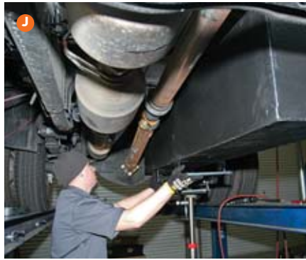
G) Soapy water and compressed air are used to double check all seals. H) Transfer Flow tank hangers hook into the factory frame slots. I) Additional padding is added on top to accommodate the shape of the larger tank. J) The new Transfer Flow tank weighs about 200 pounds, so a proper support is necessary during the installation process.
