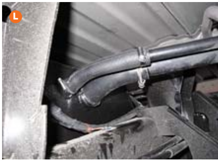
K) With the tank slightly lowered the fuel pick-up lines and electrical connection are plugged in. L) Replacement fill and vent hose connectors are supplied and need to be cut to size.
