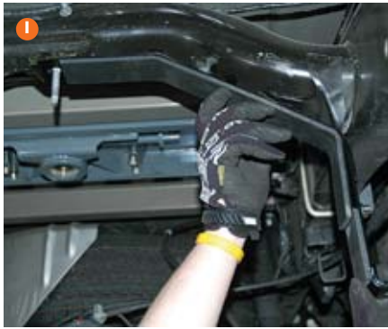
G) Soapy water and compressed air are used to double check all seals. H) Transfer Flow tank hangers hook into the factory frame slots. I) Additional padding is added on top to accommodate the shape of the larger tank. J) The new Transfer Flow tank weighs about 200 pounds, so a proper support is necessary during the installation process.
