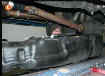
A) Though it may not look that big, the new Transfer Flow 60-gallon replacement tank for the 2012 Crew Cab Long Bed significantly extends your range. B) The first step was to loosen the short rubber connecting hoses to the metal fill and vent tubes and slip them off. C) With the factory mounting straps removed, the tank was securely supported with a hydraulic jack and lowered.
