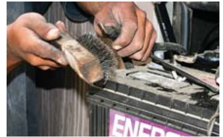
Regularly clean your battery terminals for reliability, especially after storage.
