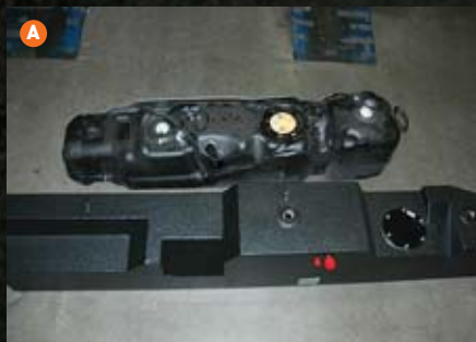
A) Though it may not look that big, the new Transfer Flow 60-gallon replacement tank for the 2012 Crew Cab Long Bed significantly extends your range. B) The first step was to loosen the short rubber connecting hoses to the metal fill and vent tubes and slip them off. C) With the factory mounting straps removed, the tank was securely supported with a hydraulic jack and lowered.
