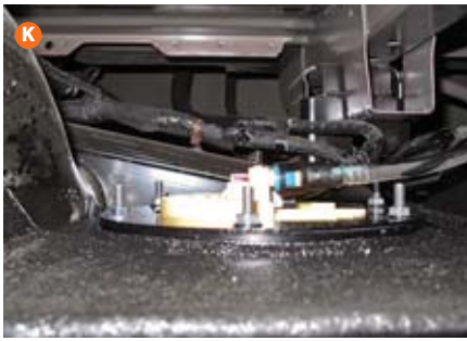
K) With the tank slightly lowered the fuel pick-up lines and electrical connection are plugged in. L) Replacement fill and vent hose connectors are supplied and need to be cut to size.
