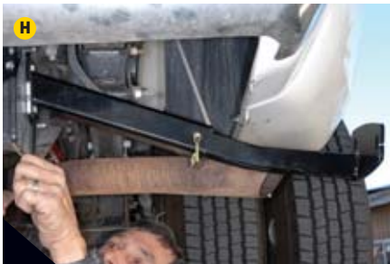
E) A piece of 3/8-inch tubing is wrapped around emergency brake line using a cable tie. F) Tubing prevents the emergency brake line from rubbing against the bracket. G) Four holes are drilled into the hitch receiver side plates. H) Rear brackets are bolted to hitch receiver side plates. Washers can be used if there's an interference problem with the exhaust tailpipe. I) Insert slides into rear bracket and is pinned in place. J) Fastgun turnbuckles must be assembled before positioning.
