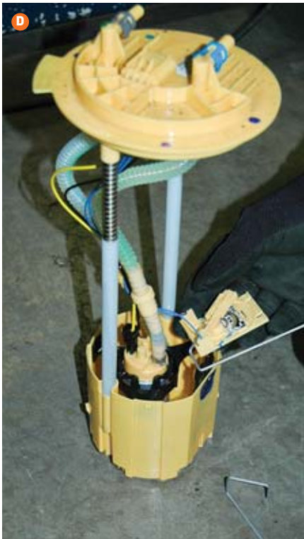
D) A new float arm was attached to give an accurate fuel level calibration for the larger tank. E) Transfer Flow replaces the twist-lock compression seal with a new O-ring and gasket, and a top-sealing ring that is attached with six nuts over studs. F) Two new rollover valves were fitted.
