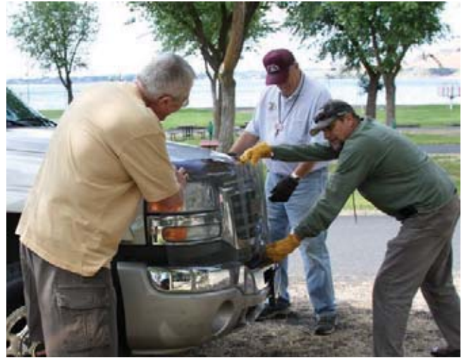
Installing a screen on your tow vehicle's grille helps keep debris off your radiator — and doubles as a butterfly-catcher.
