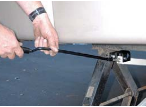
A special crank tool is used to snug the cross bars after the scissor jacks are extended. The bars are loosened so they can ride in concert with the scissor jacks and be stored close to frame (center), like the front bars (right).
