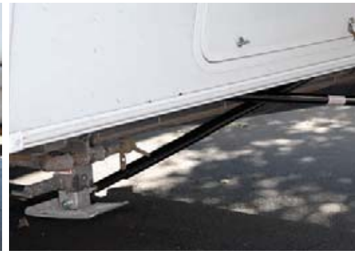
A special crank tool is used to snug the cross bars after the scissor jacks are extended. The bars are loosened so they can ride in concert with the scissor jacks and be stored close to frame (center), like the front bars (right).
