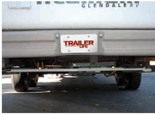
A special crank tool is used to snug the cross bars after the scissor jacks are extended. The bars are loosened so they can ride in concert with the scissor jacks and be stored close to frame (center), like the front bars (right).
