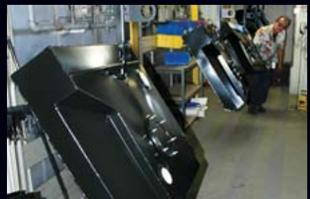
Robotic welders can make a bead to match anything done by hand. The engineering manager checks a tank for leaks with soapy water during final inspection. After final inspection, tanks are washed, dried, and powdercoated.
