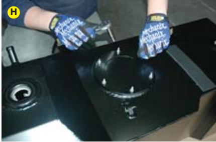
E) A single bracket is mounted to the frame using existing holes. F) Two new rollover valves were fitted. G) The OEM sending unit is reused with a new float. H) Transfer Flow used six bolts to seal the sending unit into the new tank. I) The DEF tank is not altered. J) A final step in the installation is to check and verify the calibration of the fuel level sender.
