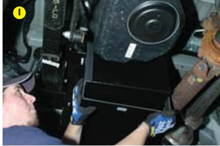
E) A single bracket is mounted to the frame using existing holes. F) Two new rollover valves were fitted. G) The OEM sending unit is reused with a new float. H) Transfer Flow used six bolts to seal the sending unit into the new tank. I) The DEF tank is not altered. J) A final step in the installation is to check and verify the calibration of the fuel level sender.
