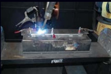
Robotic welders can make a bead to match anything done by hand. The engineering manager checks a tank for leaks with soapy water during final inspection. After final inspection, tanks are washed, dried, and powdercoated.
