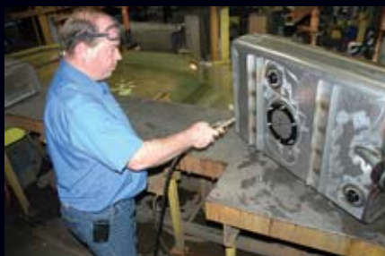
Robotic welders can make a bead to match anything done by hand. The engineering manager checks a tank for leaks with soapy water during final inspection. After final inspection, tanks are washed, dried, and powdercoated.
