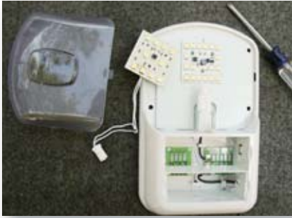
12) The Star Lights Brilliant Light fixture accepts three different power level LED cards.
