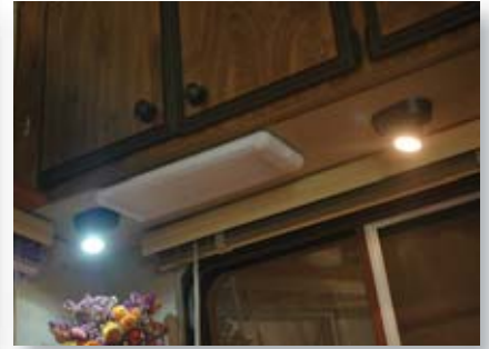
14) The Star Light replacement LED bulb, left, is clearly much brighter than the incandescent.
