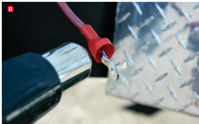
C) BlueTop batteries have SAE/automotive posts for standard battery terminals and 3/8-inch stainless-steel threaded studs that accept ring terminals. D) Cables were custom made and the ends were sealed with shrink tube that's molded into place using a heat gun. E) Batteries are connected in parallel and the cables are neatly routed, secured by tie wraps. F) Special steel pillars were built to connect the top and bottom portions of the battery box frame.
