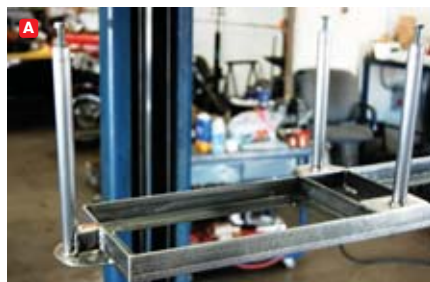
A) The battery tray is custom built using a steel framework. B) To keep weight down — and to provide protection from theft — the bottom portion of the dual-battery box frame is welded to the trailer A-frame.
