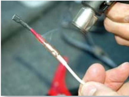
5) We used QuickCable butt connectors with built-in heat shrink for maximum reliability.
