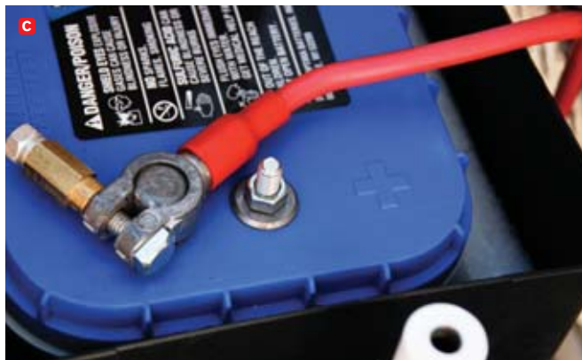
C) BlueTop batteries have SAE/automotive posts for standard battery terminals and 3/8-inch stainless-steel threaded studs that accept ring terminals. D) Cables were custom made and the ends were sealed with shrink tube that's molded into place using a heat gun. E) Batteries are connected in parallel and the cables are neatly routed, secured by tie wraps. F) Special steel pillars were built to connect the top and bottom portions of the battery box frame.
