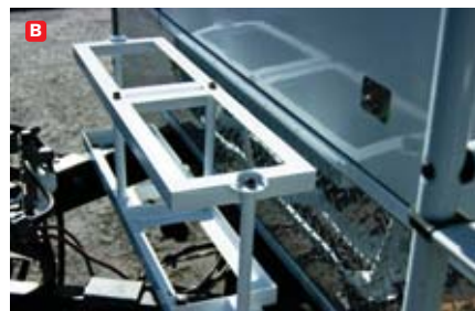
A) The battery tray is custom built using a steel framework. B) To keep weight down — and to provide protection from theft — the bottom portion of the dual-battery box frame is welded to the trailer A-frame.
