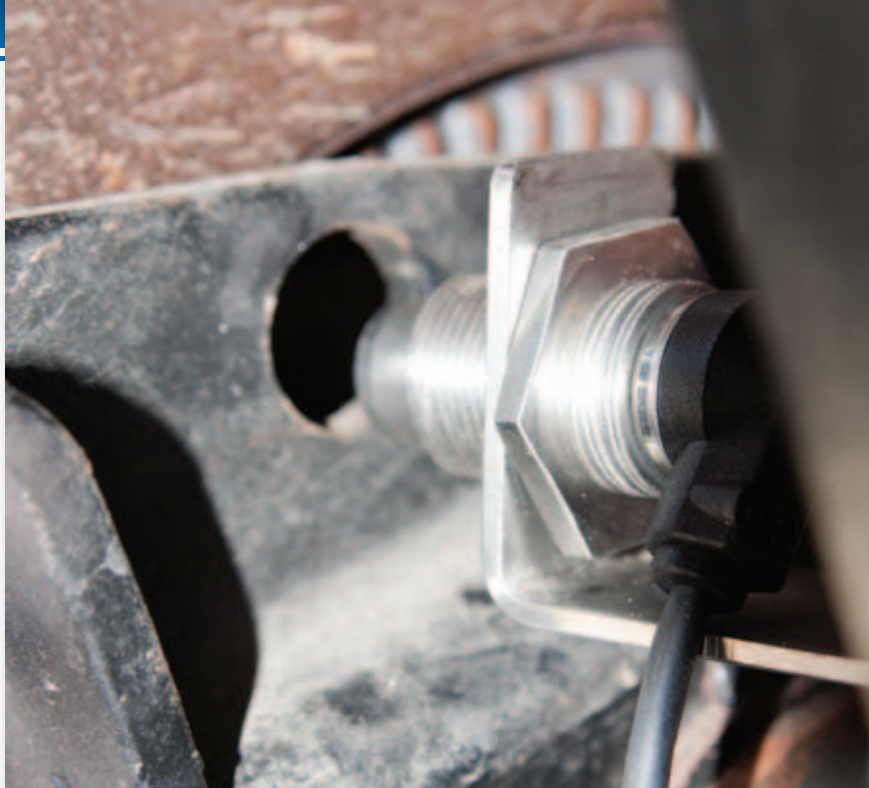
The wheel sensor is mounted on its own bracket with the spacers in place, ready to be mounted onto the brake-caliper bracket.
