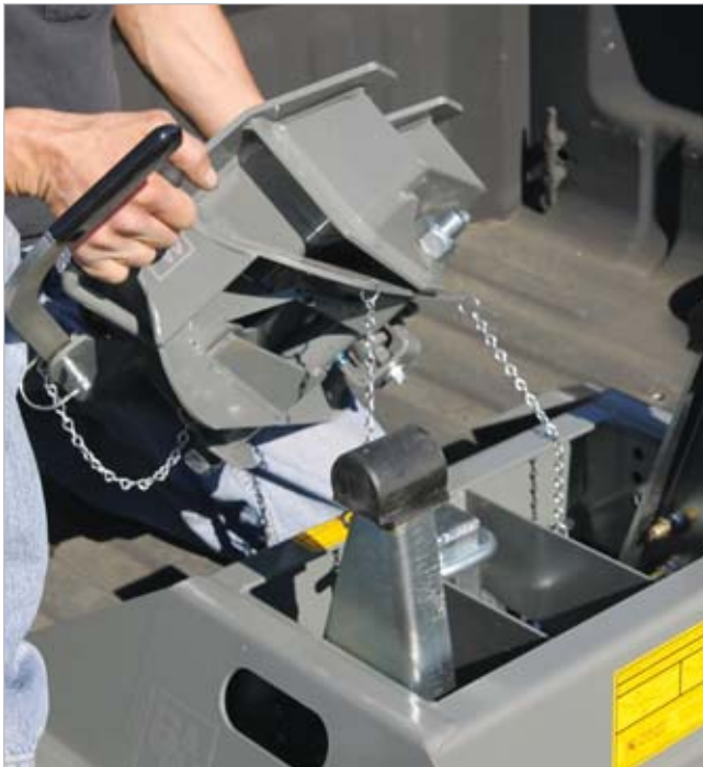
The head of the hitch easily mounts to the polyurethane rubber bushings that act as a sound dampener.
