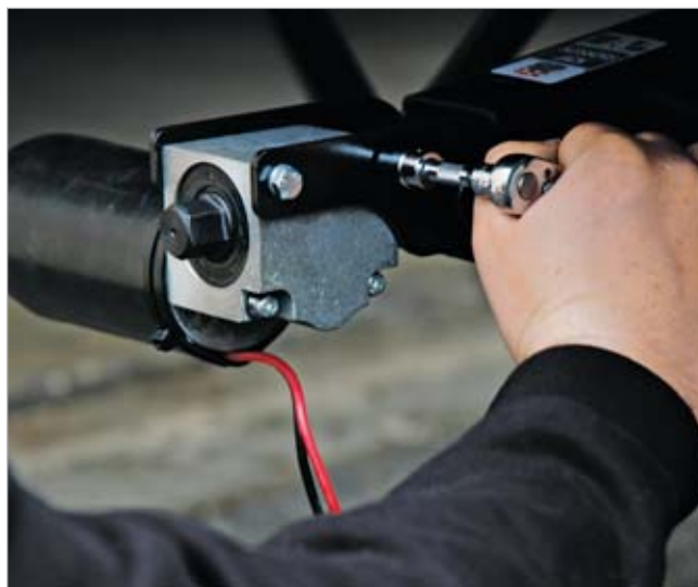
Outside brackets are attached to the motor housing using ¼-inch 20 bolts and torqued to 8 ft-lb. The fit is tight, which created a fit problem, but the issue was rectified with some grinding.
