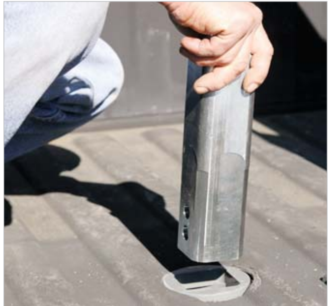
The turn-over ball is also the mounting system for the fifth-wheel hitch. So whether you are pulling a gooseneck horse trailer, your fifth-wheel, or needing the full bed of your truck for routine errands, the versatile 18K Companion Hitch makes converting from one to the other very simple.
