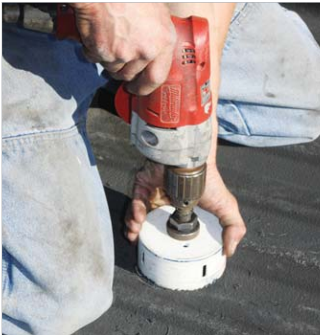
The only drilling required for the B&W hitch installation is in the bed of the truck: one 4-inch round hole for the post and four small holes where the safety chain U-bolts attach.
