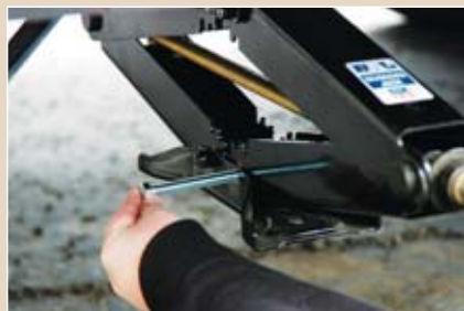
Longer bolts are used in the stabilizer foot to facilitate a location to mount the Lock-Arm bar.
