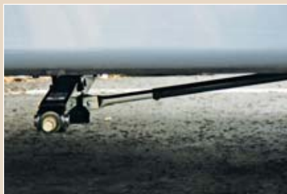
There must be a minimum of 27 inches from the stabilizers to the point where the arm attaches to the frame of the trailer.
