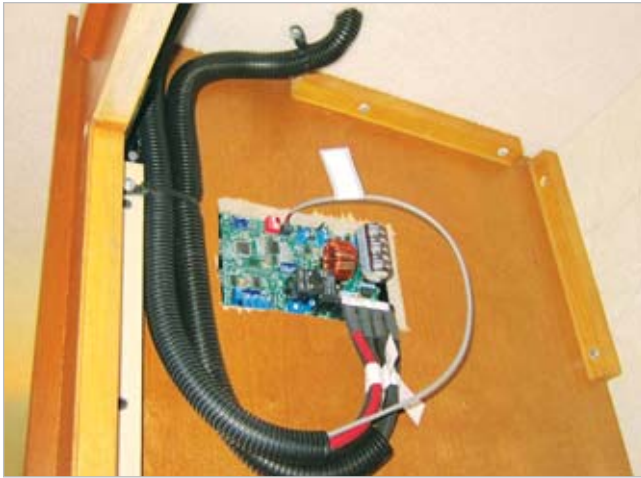
The back of the controller and the wiring loom that goes to the panels and batteries are accessible from inside the microwave cabinet. The oven was temporarily removed before installation.
