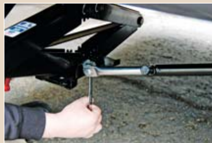
It's best to test the stabilizers by running them up and down with the arm attached before tightening the lock bolts.
