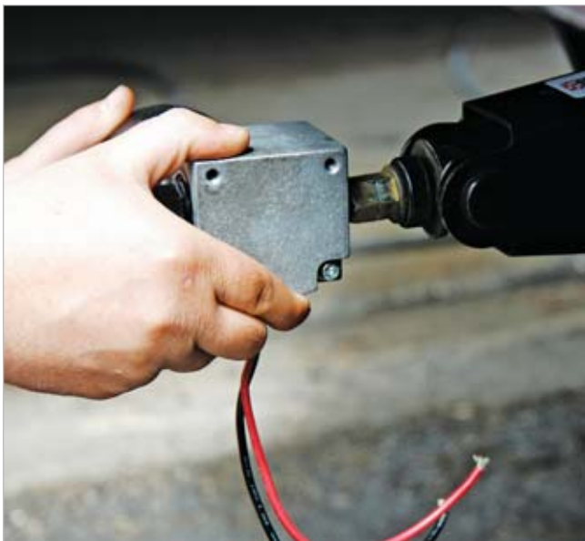
Power-Pak motors are sealed against moisture intrusion. The self-contained unit slips over the hex head (screw drive) used to manually crank the jacks up and down.
