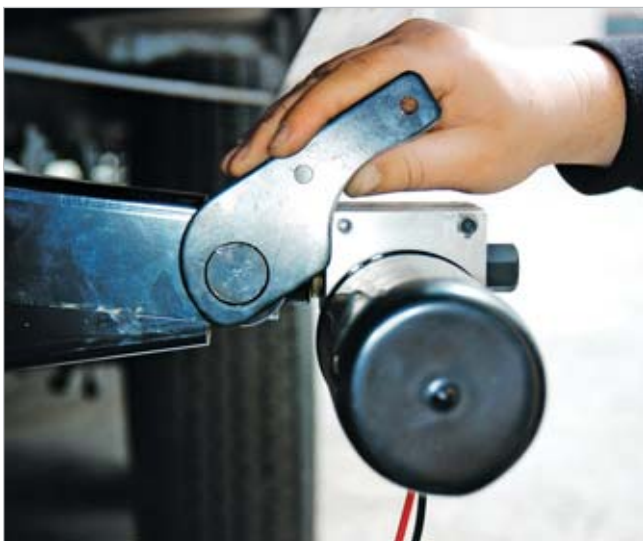
Once the Power-Pak motor is in place, the outside brackets are placed on the 1-inch trunnion before lining up with the threads in the casing.
