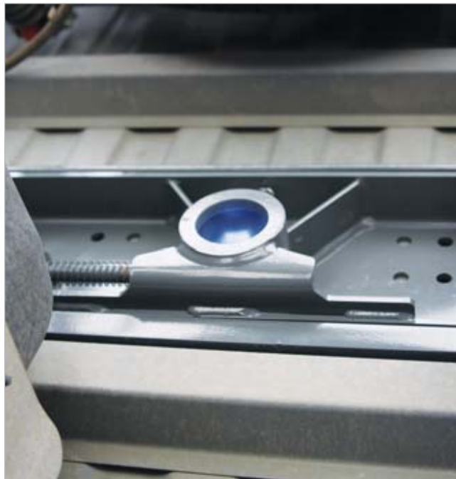
B&W's rail system mounts from underneath for an extra clean, unobstructed truck bed. The rail mounts securely without any drilling or welding to the frame.
