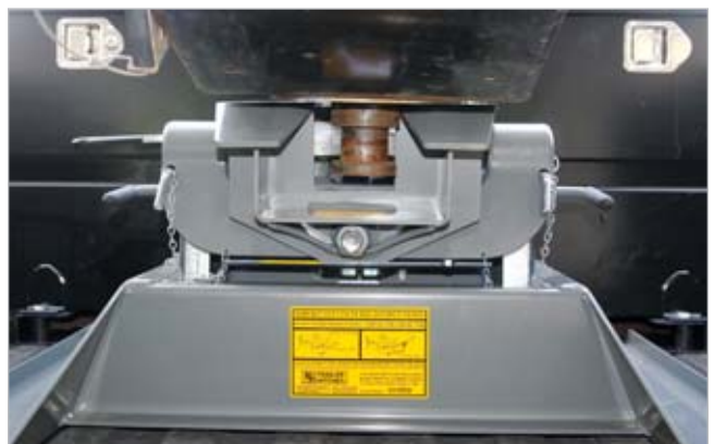
The kingpin slides into the B&W Companion wraparound jaws.
