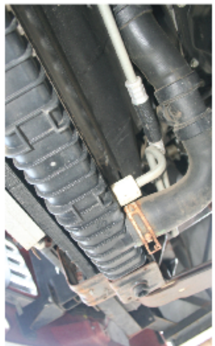
This type of hose clamp is prone to rust and breakage — replace with stainless steel clamps.
