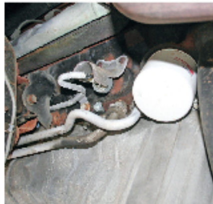
The oil filter (on the right) is often tucked away in a spot that is difficult to reach.
