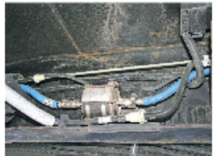
Fuel filters are often hidden within the frame rails and are easily overlooked.
