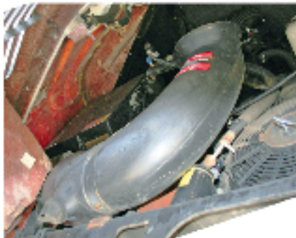
Check air inlet tubes for leaks, mounting security and damage.
