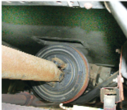
Check U-joint mounting fasteners and items such as exhaust hangers (on the right) for wear.
