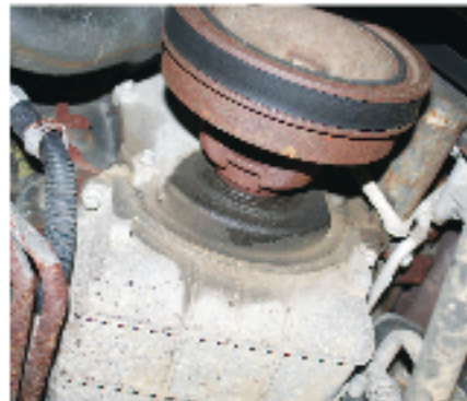
Check for oil leaks; this front seal is just starting to seep.
