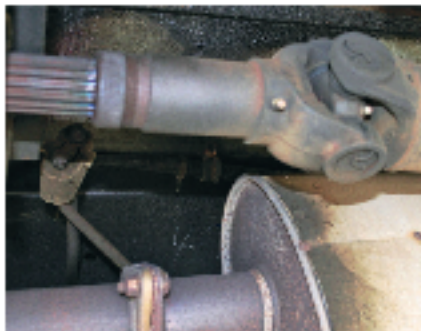
U-joints and slip yokes need to be greased and inspected for looseness and wear.
