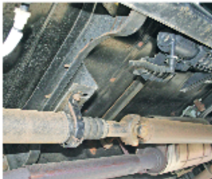
Check driveline hangers for cracked and damaged rubber, and bearings for wear.
