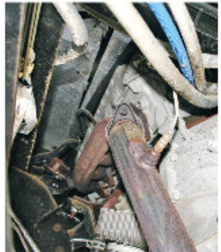
Oxygen sensors are mounted in the exhaust pipes and need to be checked.
